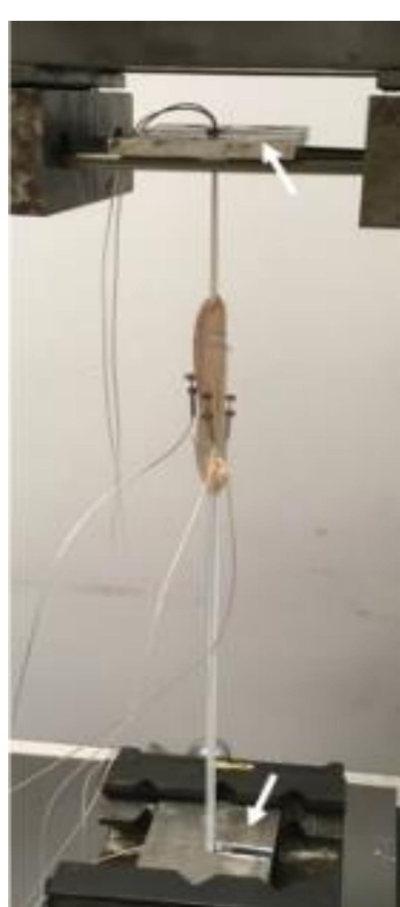
Figure 1: Tension test of the constructs, left. Right, 1 matched pair showing the effect of inner band slippage in black UST v red SST.
