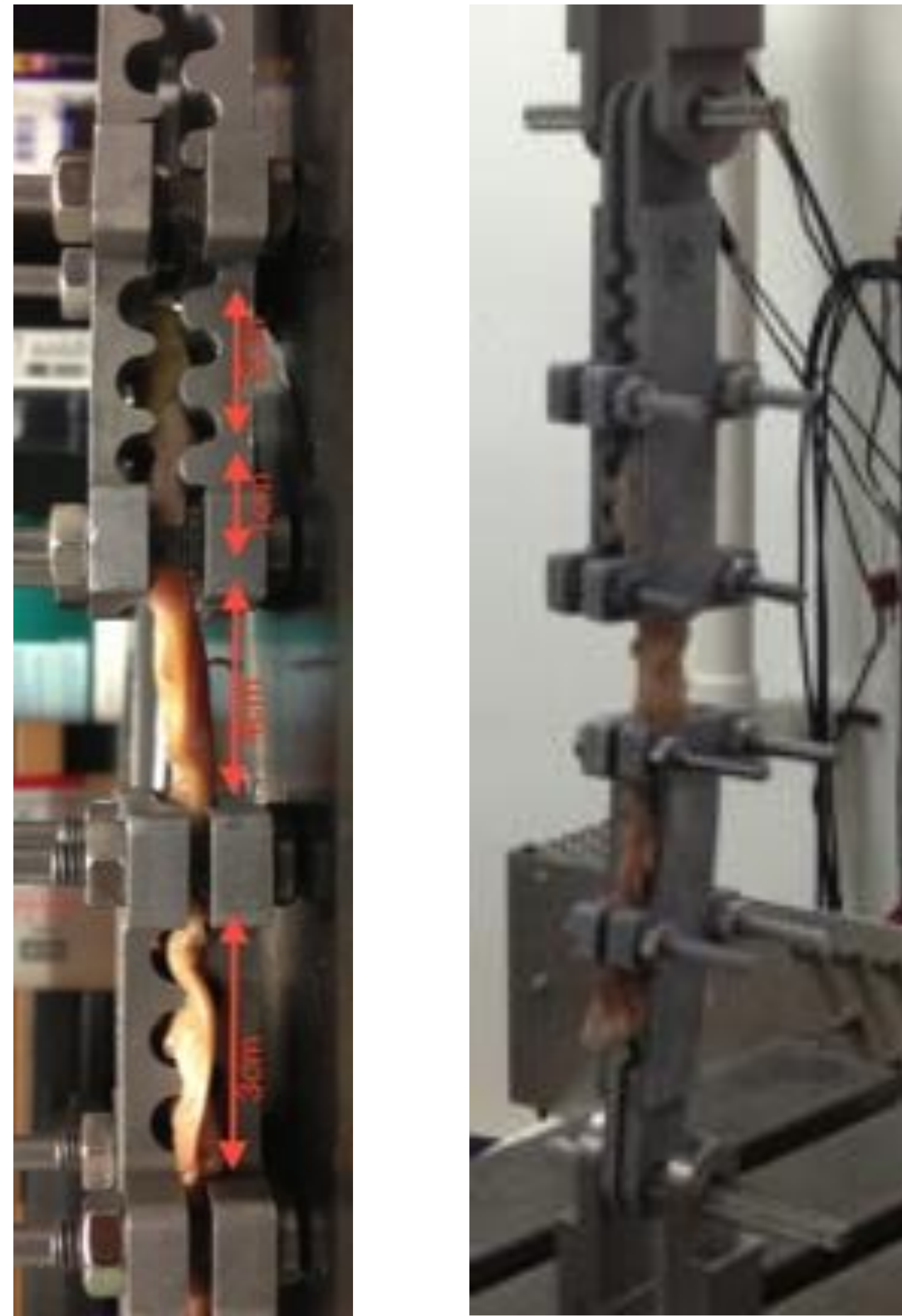
Figure 2 Specimens were mounted with a 4 cm working length, left. The grips were frozen and the specimen pulled at 100% strain/second, right.
