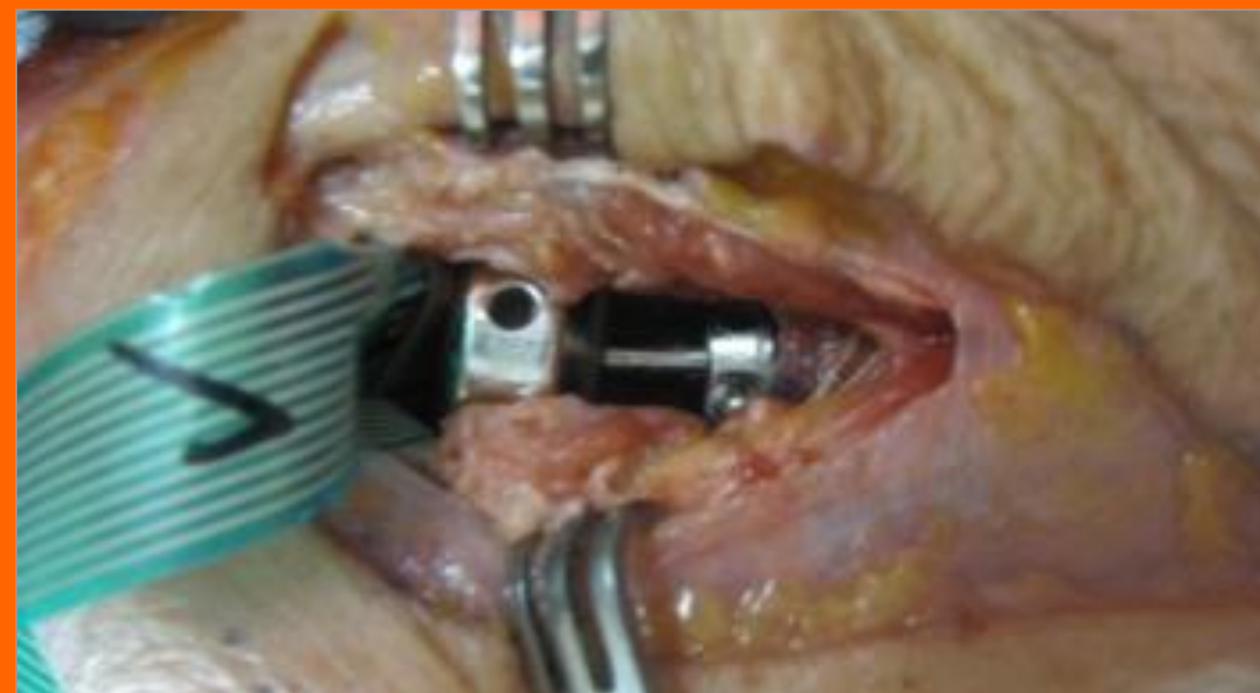
Figure 2: The radial head implant placed against the capitellum with the Tekscan transducer in between to measure the contact pressure.
