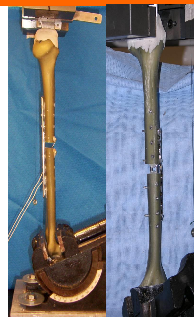
Figure 2 – setup for flexion and axial torque loading. Note LED's for measuring movement across the gap.
