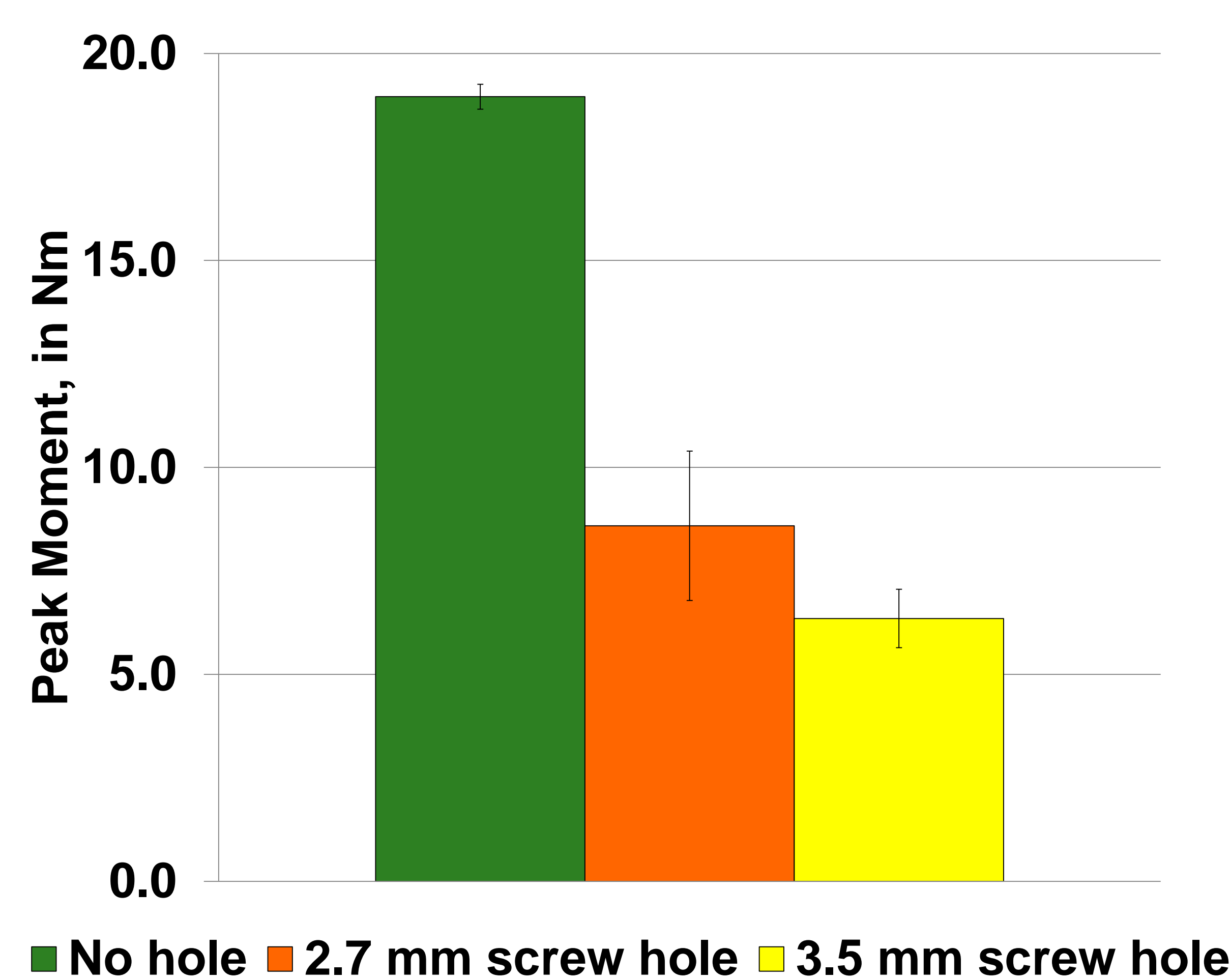
Figure 2 – The 3.5 mm screw holes weakened the bone model significantly more than the 2.7 mm screw holes in bending.
