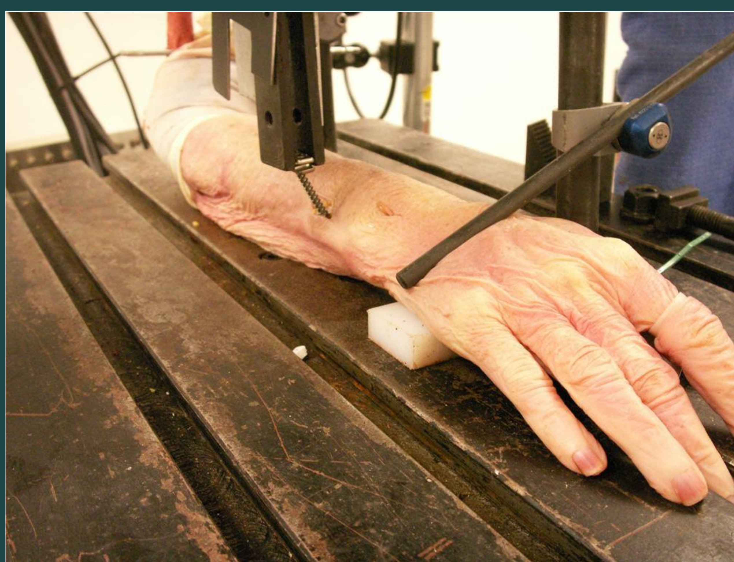
Figure 2: Testing set up with carpals locked and the distal ulna translated by the MTS through a polyaxial bone screw.
