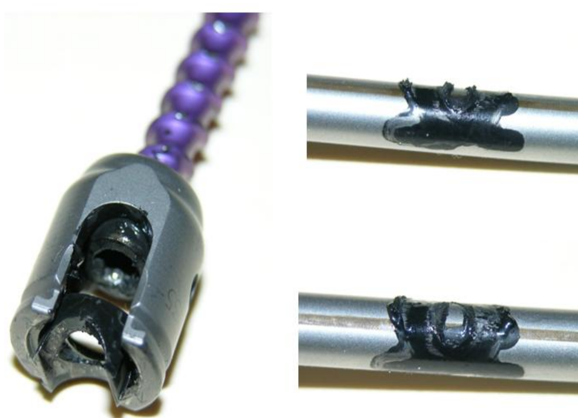
FIGURE 3– Wear Debris from testing 150,000 cycles
