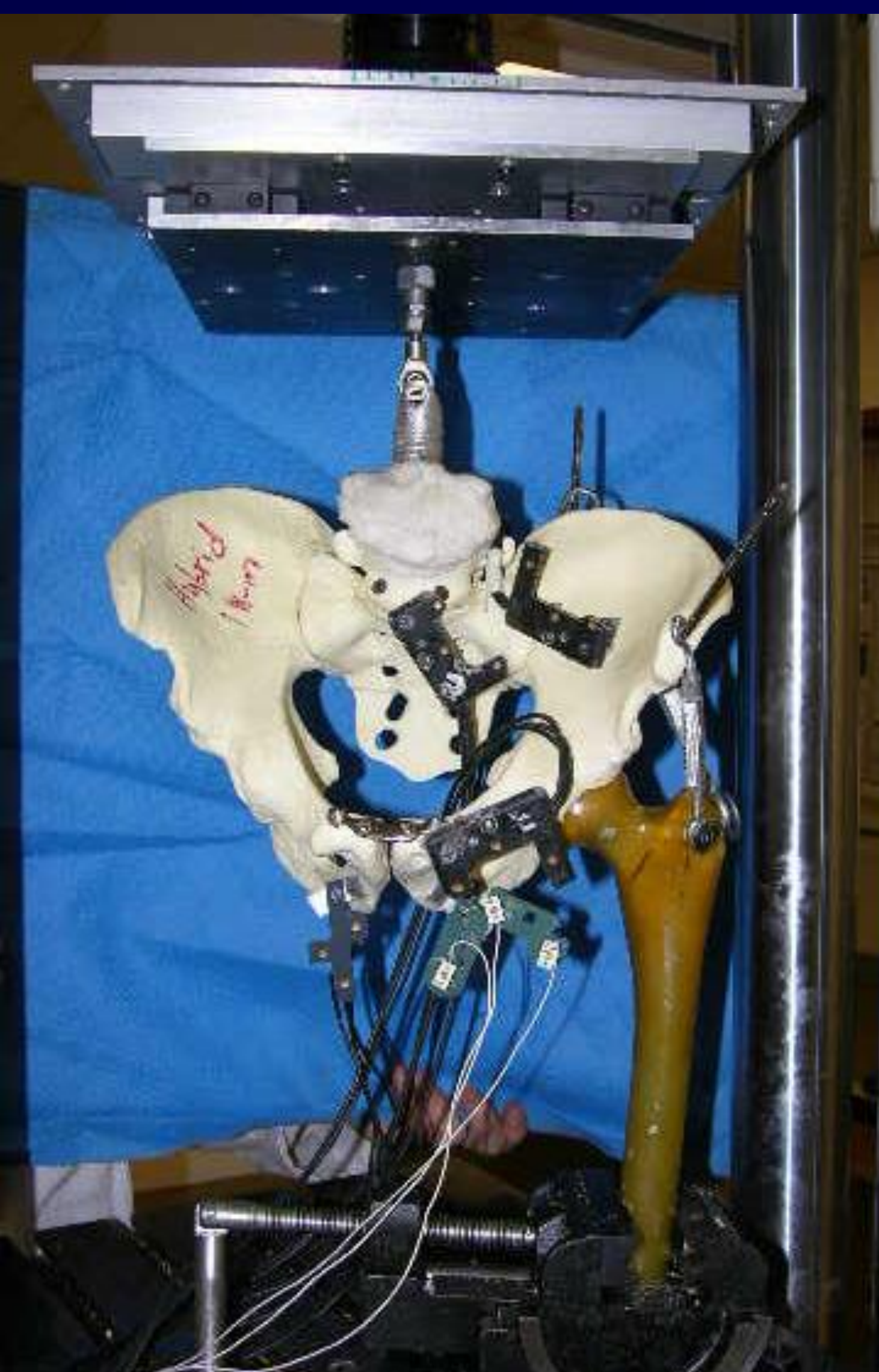
Figure 1 – AP view of the pelvis with the MTS applying a vertical load through linear bearings to assure the load follows the movements of the pelvis as it rotates on the femur in simulated single leg stance loading. The femur is adducted to 8 degrees with the abductor force simulated through the turnbuckles. The LED brackets measure the 6 DOF motions of each bony part.
