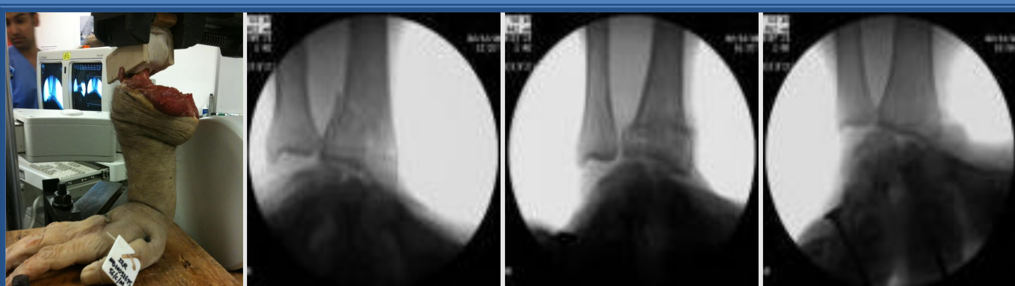
Figure 2: (Color image) 5N-m external forearm rotation ulnarly deviated 10-15° (Fluoroscopy images) Examples of distal radius fractures sustained.
